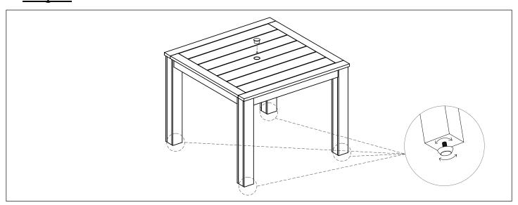
Using a second person to assist you, turn assembly upright. Assembly is now complete and the product is ready for use. Adjustable levelers are located on the bottom of each leg and may be adjusted by turning outwards, counter-clockwise to help account for uneven surfaces. NOTE: Hardware may loosen over time. Periodically check that all connections remain tight and adjust as needed. Insert Parasol Cap (C).
