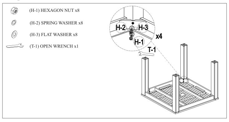
Place Table Top Panel (A) upside down on a padded non - marring surface. Insert bolt on Leg (B) through predrilled holes in corner of apron. Secure bolts with Flat Washers (H-3), Spring Washers (H-2) and Hexagon Nuts (H-1), stacking the hardware in the order as shown. Loosely install hardware on both bolts. Fully tighten using Open Wrench (T-1) after all hardware is installed. Repeat for remaining Legs (B).
